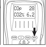
Press "Send" to print results or press and hold "Send" to log results from any screen.
