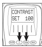
Press "▲" UP or "▼" DOWN to adjust screen contrast. NOTE: The higher the value the lighter the digits appear
