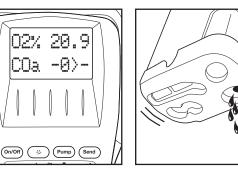
Remove the probe from the flue and allow the analyzer to purge with fresh air until readings return to zero. - 02 to 20.9%, CO to Zero (Be careful as the probe tip will be HOT)
