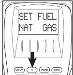
Rotate test selector to **Fuel**.
