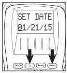
Date displays with the cursor underneath the first digit. Press "▲" UP or "▼" DOWN to increase or decrease and press ENTER "←" to set and proceed to next digit.
