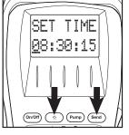
Clock displays with the cursor underneath the first digit. Press "▲" UP or "▼" DOWN to increase or decrease and press ENTER "←" to set and proceed to the next digit.
