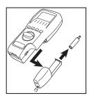
This is a very important part of the analyzer and should be changed regularly. It prevents dust and dirt particles from entering the pump and sensors that will cause damage. The filter MUST be changed when it appears discolored on the inner surface.
