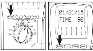
Power on in area of fresh air and allow to countdown. On sealed combustion appliances (ducted inlet) connect flue probe and power on outside and allow to continue to set inlet temperature. (see page 12)
