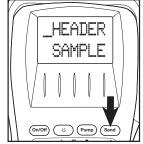
The existing HEADER 1 will display with the cursor underneath the first digit. Press "▲" UP or "▼" DOWN to change and press ENTER "←"" to set and continue to the next digit. Press ENTER "←"" to proceed.
