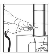
Insert Flue Probe in stack. Adjust the cone so the end of the probe is approximately at the center of the stack (4" stack adjust cone to approx. 2" from end of probe.)
