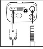
Connect flue probe thermocouple connector to T1, and connect flue probe to water trap as shown above.
