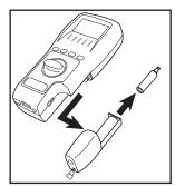
Check particle filter for dirt and any other sediment and replace if necessary.
