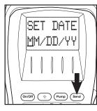
Set date displays with MM/DD/YY Press "▲" UP or "▼" DOWN to select a different format press ENTER "← " to proceed. Use MM/DD/YY for North American.
