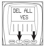
Press "▲" UP or "▼" DOWN to select Yes or No Press ENTER "← " to proceed. Analyzer will automatically return to the menu.
