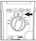
Rotate selector to desired test.
