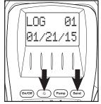
Press and hold "▲" UP or "♥" DOWN to select log to view (LOG 01, LOG 02). Press "▲" UP or "♥" DOWN to scroll and view parameters on second line.
