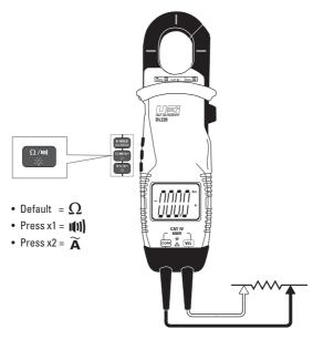
• Buzzer sounds at less than 40  $\!\Omega.$
