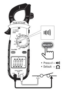
Buzzer sounds at less than  $40\Omega$ .
