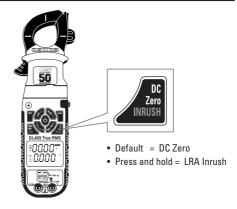
The UEi LRA Inrush is programmed to properly capture the starting current for compressor motors.
