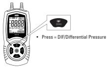
**NOTE:** Prior to use the Manometer must be zeroed. To do this. ensure the Manometer is in a non-pressurized area and no hoses are connected. The Manometer has a 10 second count down upon powering on.
