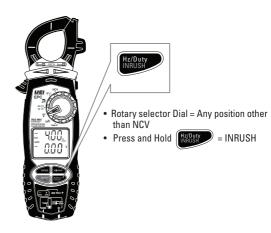
The UEi LRA Inrush is programmed to properly capture the starting current for compressor motors. Inrush current can be measured in any position of the rotary selector Dial.
