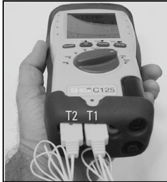
Connect flue probe thermocouple or accessory thermocouple connector to T1. Connect accessory thermocouple probe to T2. Compatible with any K-Type thermocouple.
