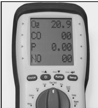
Rotate selector to "Flue Test" and begin testing.
