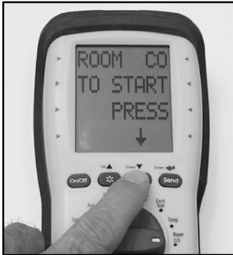
Disconnect all probe connections from the C125 and place handset in the area to be tested. Rotate selector to Room CO
