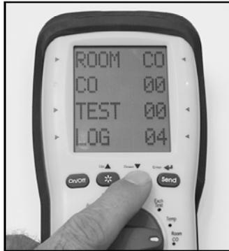
Press the PUMP button to start the test. The CO reading will be logged every 2 minute for 30 minutes and store a summary that can be printed.
