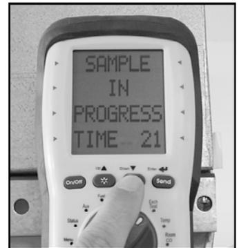
The meter will wait 30 seconds and then record the values for CO, O<sub>2</sub> and Excess Air. Test results will automatically be stored and include the values before the blower turns on, the values after and any variance. View or print these values from the Report menu.
