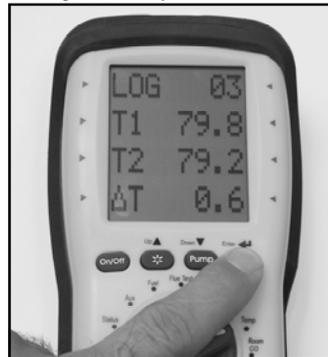
Press and hold "SEND" to log the current readings for Combustion Flue Testing, Pressure (draft) Differential, and Temperature selector positions.
