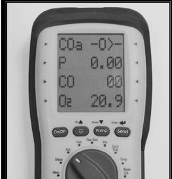
The display on the AUX setting can be customized to any four parameters you choose. These are selected on the MENU selector, scroll to SCREEN, scroll to AUX then select Line 1 through 4 and choose the desired measurements. Note: CO Air Free is only available on the AUX screen.
