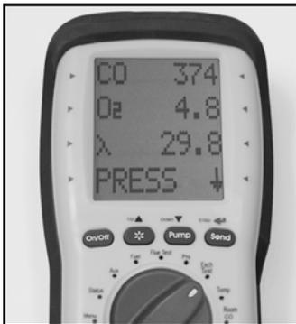
Rotate selector to Exch Test. Call for heat on the furnace. Observe the levels for O<sub>2</sub> and CO.
