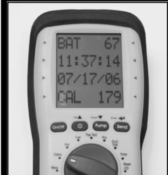
The status page provides a quick overview of the remaining battery life, currently set date and time, and the number of days remaining until the recommended calibration schedule.
