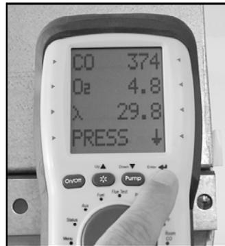
Prior to the blower turning on, and when the O<sub>2</sub> readings have stabilized press the SEND button.
