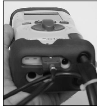
Connect flue probe thermocouple connector to T1, and connect flue probe to water trap. Use optional probe with T2 for inlet temperature.
