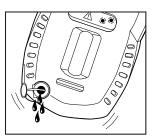
Remove the rubber boot and red drain plug. Allow the water to drain out. Re-insert the rubber plug and replace boot cover.
