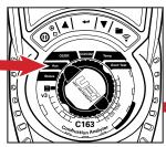
When performing a combustion Test, Rotate function rotary dial to AUX to view the Auxiliary Test Screen's custom parameters.
