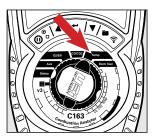
Rotate function rotary dial to TEMP for Temperature Test Screen.
