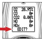
AUX displays 5 lines of editable parameters. To edit line values Press ▼ button until **Edit?** displays on the Status Bar. Press and Hold ← until the
