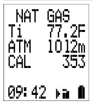
*Current fuel selection. Use status bar to change fuel selection.* Select between: Pellets, Light Oil, Heavy Oil, LPG, Butane, Propane, Natural Gas, Bio Oil
