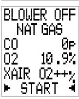
In Blower Off mode, Press 🕶 to start test
