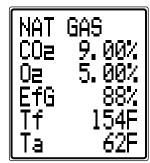
Fuel type can be changed via "MENU" or "STATUS" setting. Carbon Dioxide (%) Oxygen (%) left after combustion. Should be  $20.9\% \pm 0.3\%$  in fresh air. Gross efficiency Flue temperature (°F). Inlet temperature (°F). Normally set by flue probe during fresh air purge.
