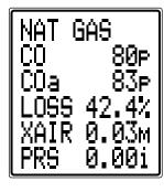
Fuel type can be changed via "Menu" or "STATUS" setting. Carbon monoxide (ppm).
