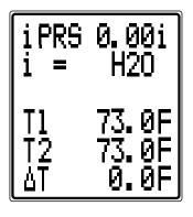
Pressure units can be selected via "MENU". Eg Flow Temp Eg Return Temp Differential Temp
