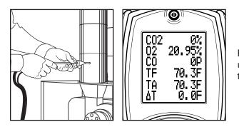
Remove the probe from the flue and allow analyzer to purge with fresh air until readings return to zero. 02 to 20.9%, CO to Zero (Be careful the probe tip will be HOT).
