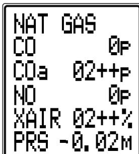
The NO readings are printed and stored in the same way as the other combustion gas readings. On the printouts the NO readings appear directly below the flue CO readings. OR AUX
