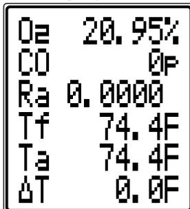
The AUX (auxiliary) display can be customized via MENU / SCREEN / AUX. The parameters displayed on lines 1, 2, 3, 4, 5 and 6 can be set by the user. They remain the AUX parameters until changed by the user.
