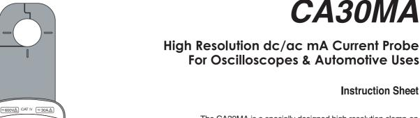
The CA30MA is a specially designed high resolution clamp-on DC/AC mA current adapter. This probe will allow your oscilloscope /multimeter to measure low current up to 30 A with 1 mA resolution and an accuracy of 1%. With this clamp there is no need to break the circuit as is typical with digital multimeters or other low current measurement techniques.
