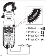
• Buzzer sounds at less than <  $40\Omega$ .
