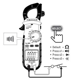
Buzzer sounds at less than 40Ω.
