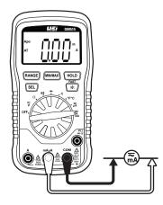
Keep hands behind test lead guards when measuring current levels.
