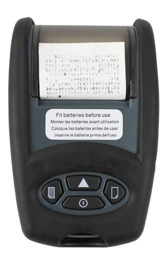
The IRP-2 is a portable printer using thermal paper that links to other UEi products using an infrared link. It incorporates an 'easy load' paper facility and allows NiMh batteries to be recharged in situ.
