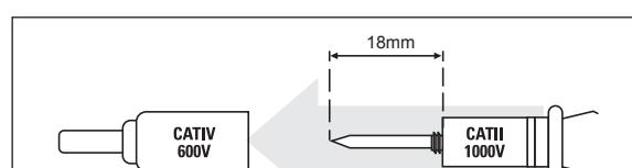
• CAT IV shields may be removed for CAT II locations. This will allow testing on recessed conductors such as standard wall outlets. Take care not to lose the shields.
