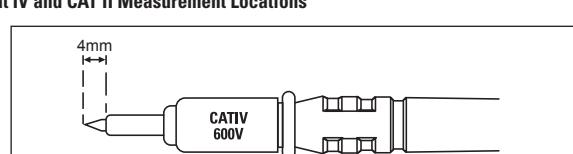
• Ensure the test lead shield is pressed firmly in place. Failure to use the CAT IV shield increases arc-flash risk.
