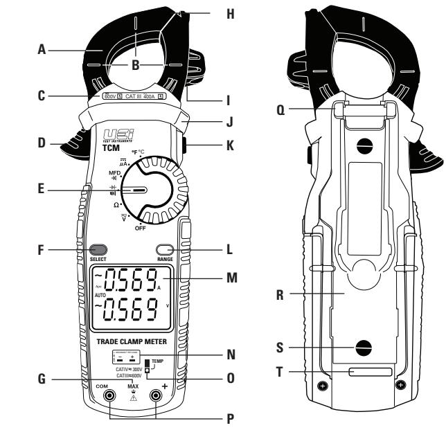
**A. Clamp:** Measure inductive AC current. Opens to 1.26" (32.0mm).
