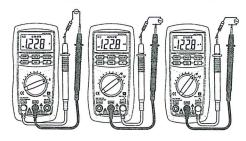
4.12.1 Connect the black test lead to the COM jack and the red test lead to the INPUT jack for a maximum of 200mA current. For a maximum of 10A, move the red lead to the 10A jack.
